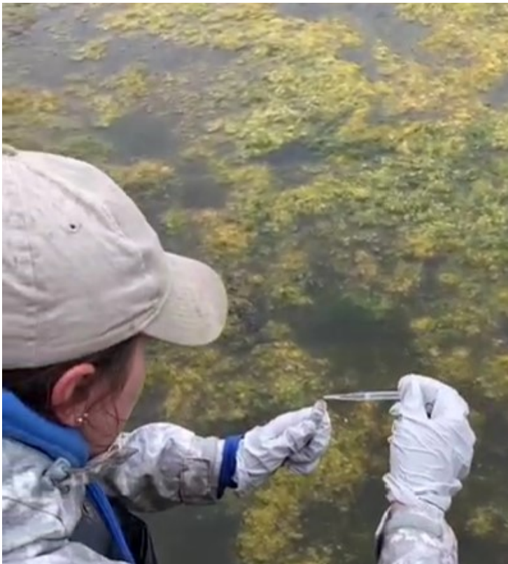
Using a cyanotoxin test kit on a surface bloom last year
