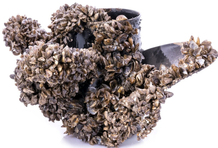
Zebra mussels encrust a boat propeller
